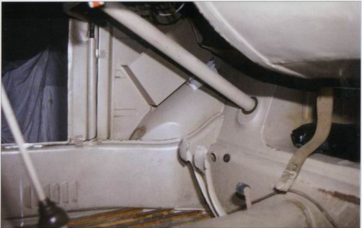
Air vents below door are a part of heating system and lead the warm air from the engine compartment to the cab. Heating has, however, very low efficiency and the warm air is hardly able to warm up the driver's boots. Note also the sheet metal box for storing documents located on the body side left to the steering column.
