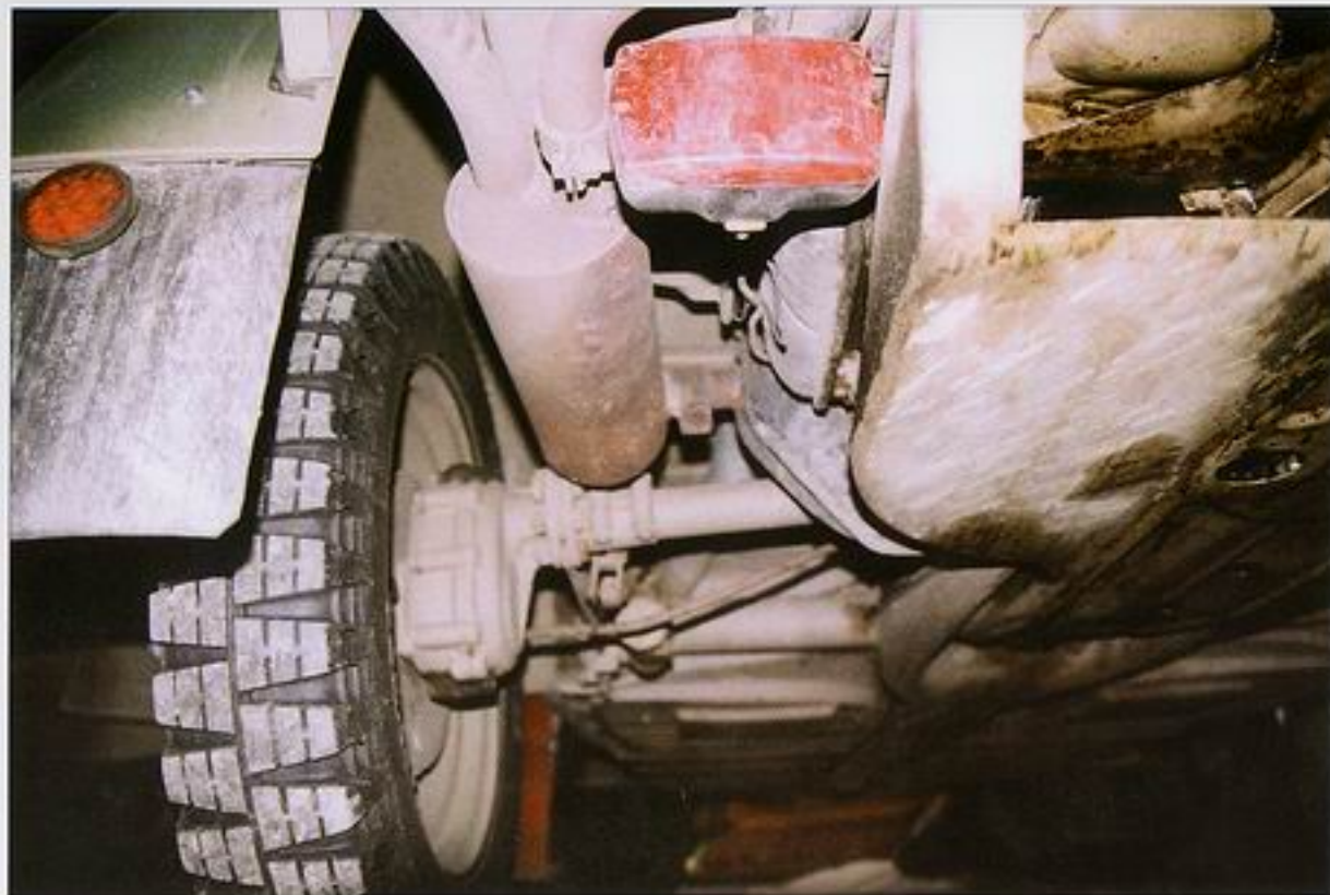
Top and bottom left pictures show frog view of the rear part of the body and engine. There are two exhaust silencers, one on each engine side. Left silencer tube is connected with injector sucking dust and sand from centrifugal filter installed on air intake.
