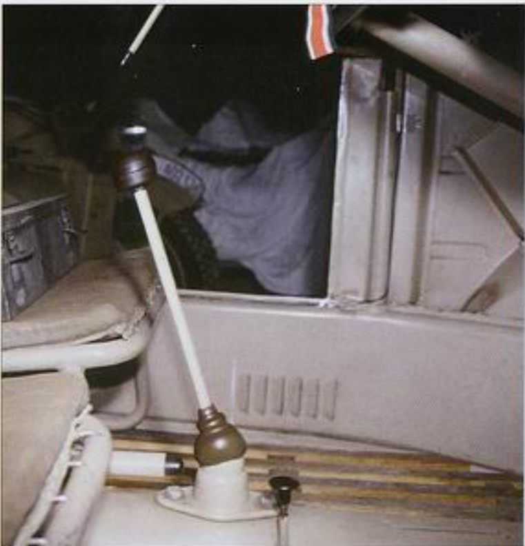
Air vents below door are a part of heating system and lead the warm air from the engine compartment to the cab. Heating has, however, very low efficiency and the warm air is hardly able to warm up the driver's boots. Note also the sheet metal box for storing documents located on the body side left to the steering column.
