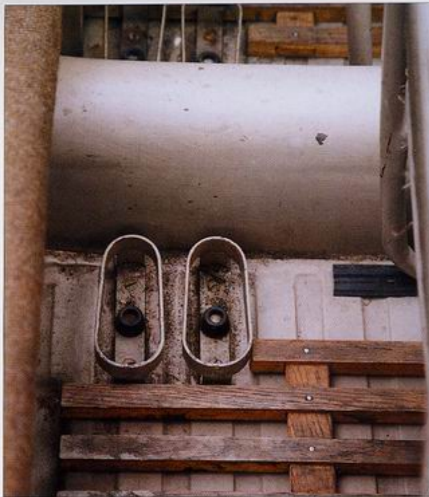
Lower left picture shows detail of the fuel cock and its protection against breakage.
