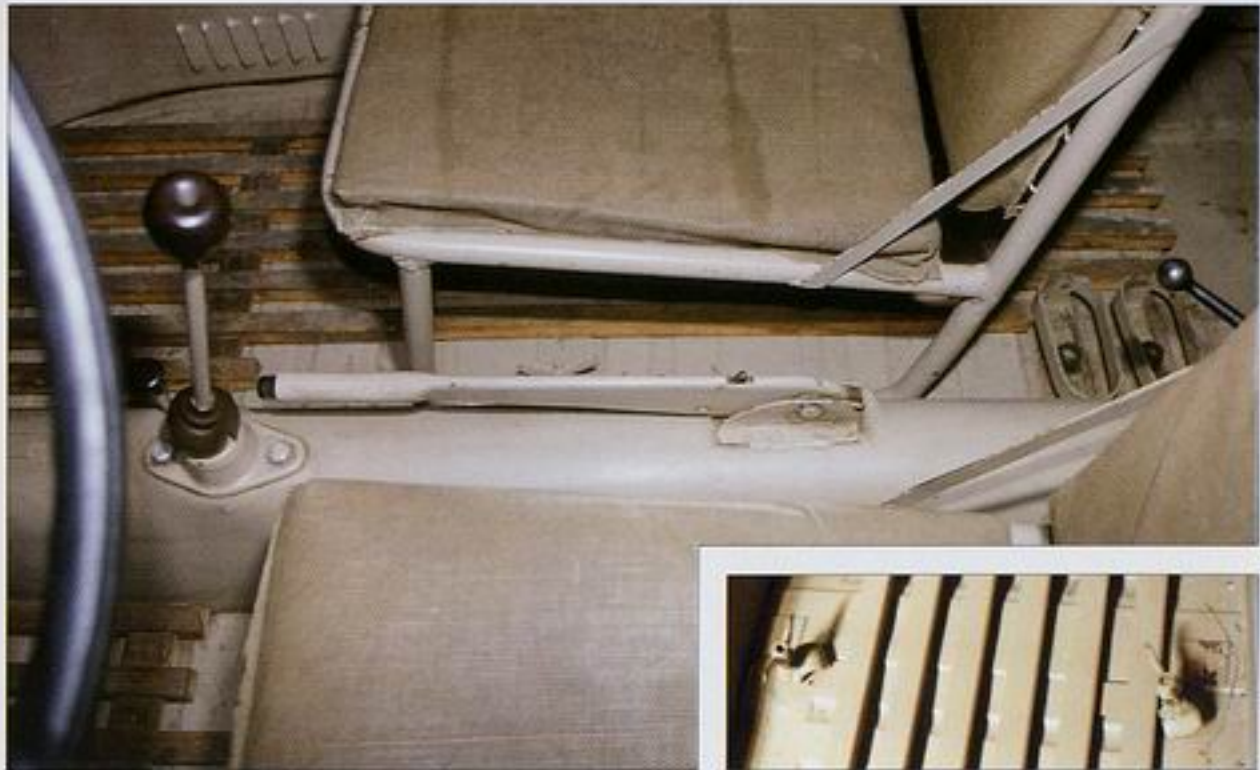
KdF is equipped with mechanically operating brakes. Manual parking brake is mechanically connected to service brakes and controls the brakes by means of steel cables. the small picture on the right shows wingnuts and brackets used for fixing front seats on the floor.
