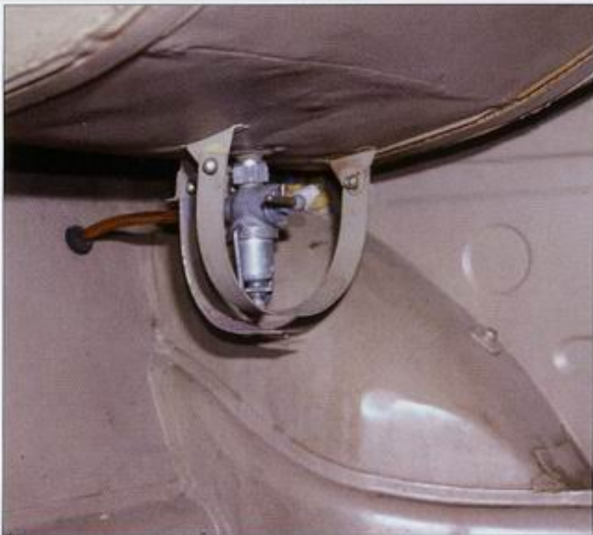
Lower left picture shows detail of the fuel cock and its protection against breakage.
