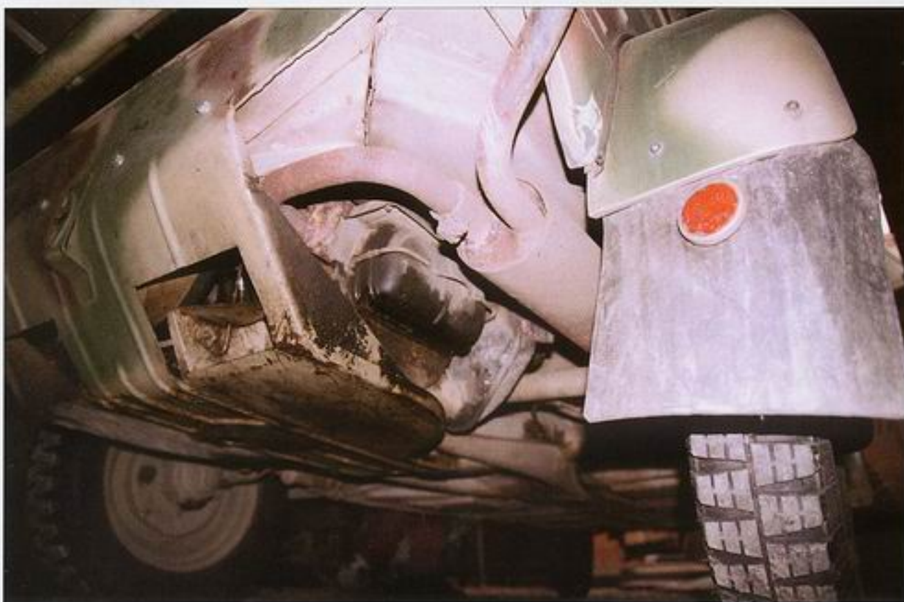
Top and bottom left pictures show frog view of the rear part of the body and engine. There are two exhaust silencers, one on each engine side. Left silencer tube is connected with injector sucking dust and sand from centrifugal filter installed on air intake.
