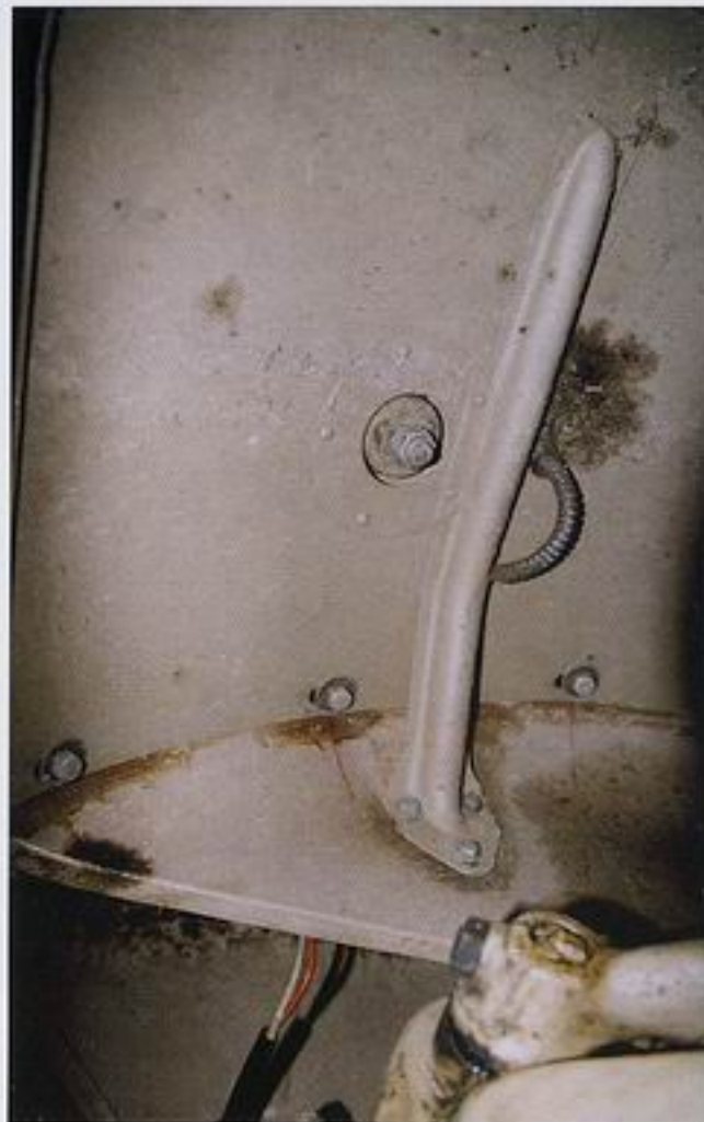
Front mudguards are reinforced by pressed brace shown on the picture above in frog view.
