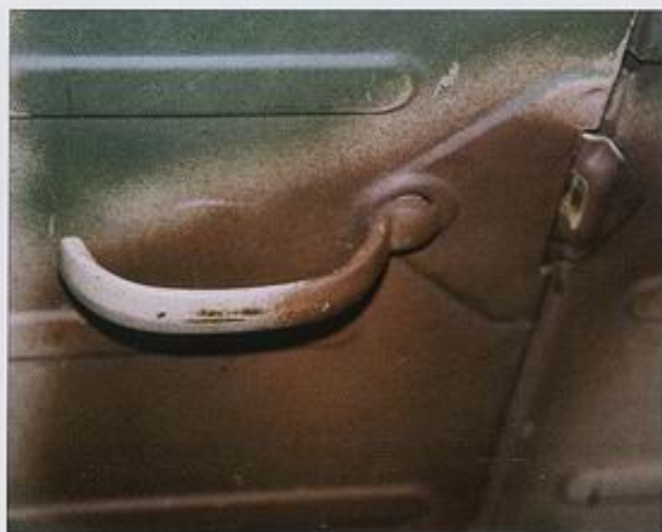
Detail of external door handle is shown on the picture above. The handles themselves were the same like internal ones.
