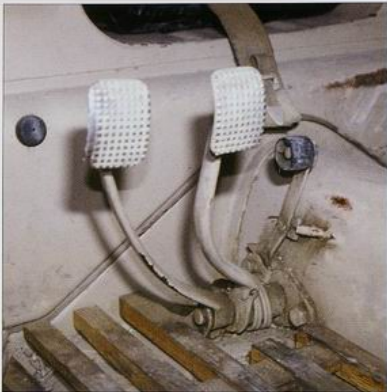
Picture above shows the installation of clutch, brake and accelerator pedals. Bakelite roller on the top of accelerator pedal improves the throttle actuating when driving in rough terrain.
