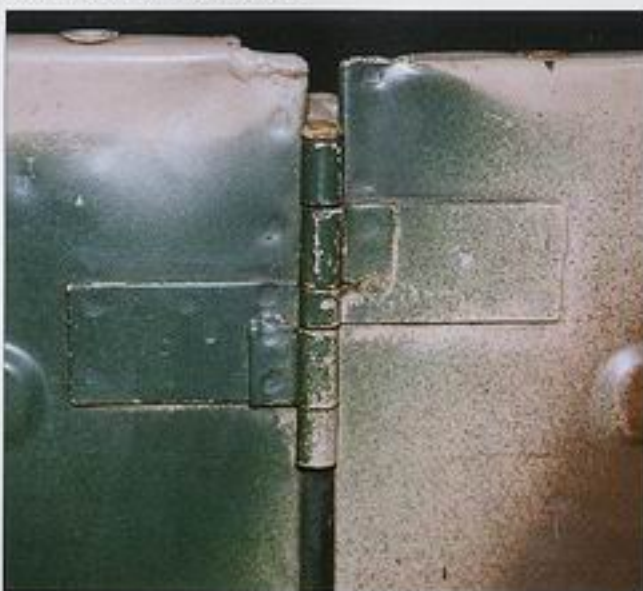
Picture above shows the cab door hinge, viewed from inside.
